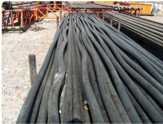
Figure 5—A high pressured, fracture treatment allowed the pipe to buckle. A permanent deformation of the pipe occurs when the buckling-induced stresses exceeds the pipe's yield strength. (Photograph courtesy of Dr. Robert Mitchell.)
