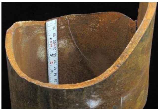
Figure 9—A visual examination of the failed casing showed a brittle fracture. Lab testing indicated that the failed specimen's yield strength exceeded the API's acceptable ranges. The pipe was improperly tempered during the manufacturing, as shown by harness testing. (Case History No. 10)
