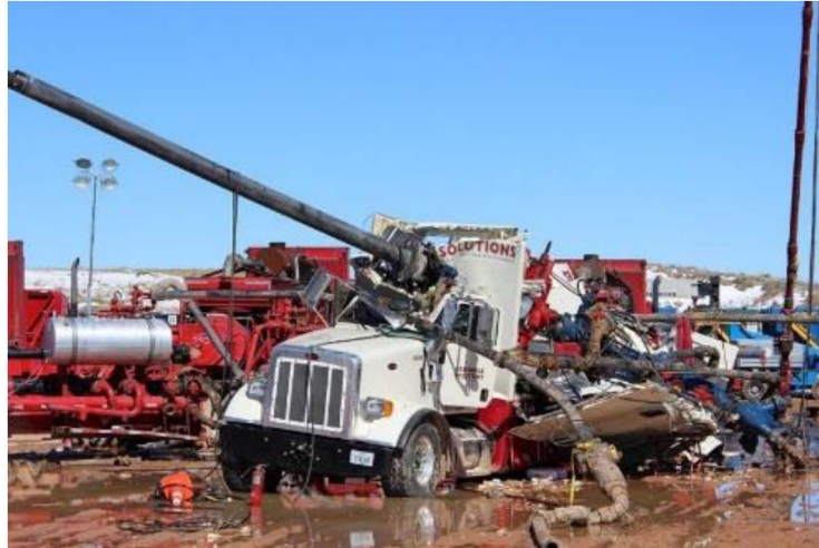
Figure 10—A crack at the wellhead-casing interface caused this failure (see Table 2, number 4). The wellhead and short sections of surface and production casing were ejected. The projectile speared the truck's cabin. (The driver was not in the truck.)
