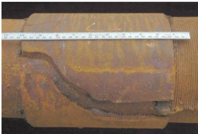
Figure 8—The crack observed in this photograph resulted from coupling fatigue. (Case History No. 7)
